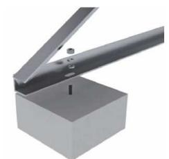
Triangle structures are connected to concrete bases by bolts.
