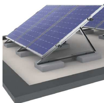
Fix the aluminium rail to the triangle structure by adopting T-head bolts.
